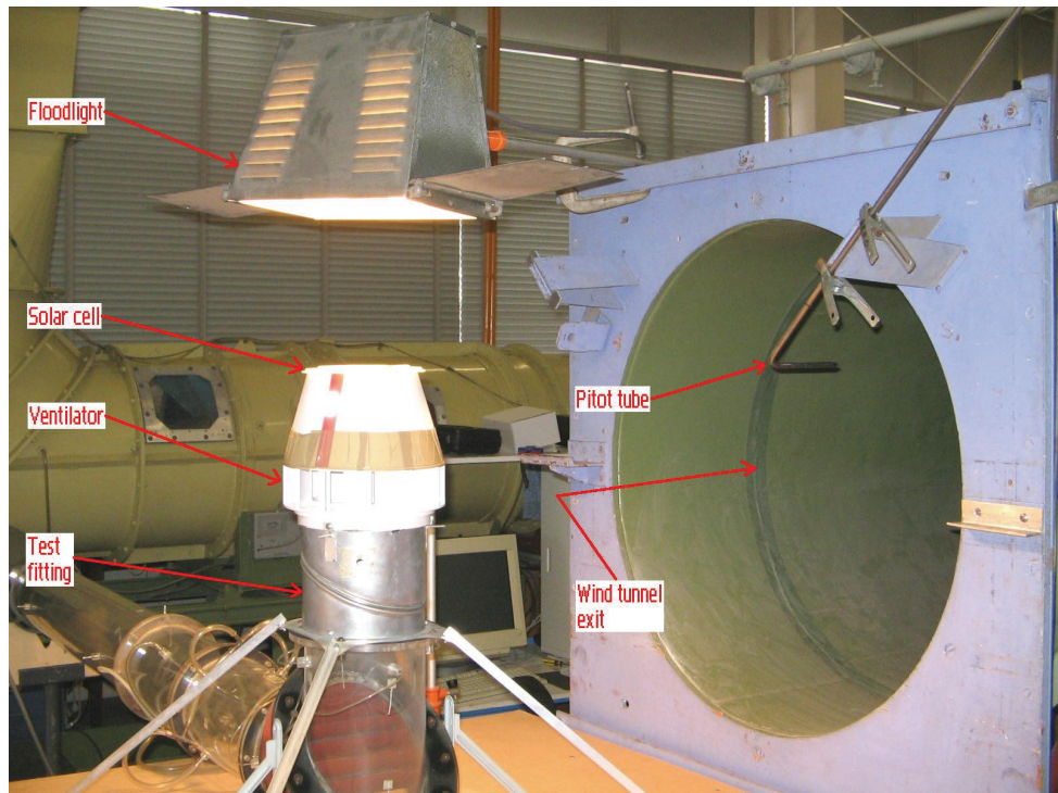
Fig. 12. Test set-up of wind-solar hybrid ventilator
