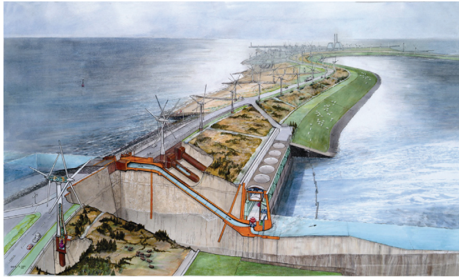
Fig. 16. Artist impression of the Energy Island with an Inverse Offshore Pump Accumulation (IOPAC)
