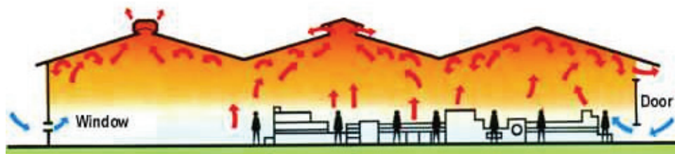
Fig. 1. Ventilation by Natural Convection (Image: www.lomanco.com )
